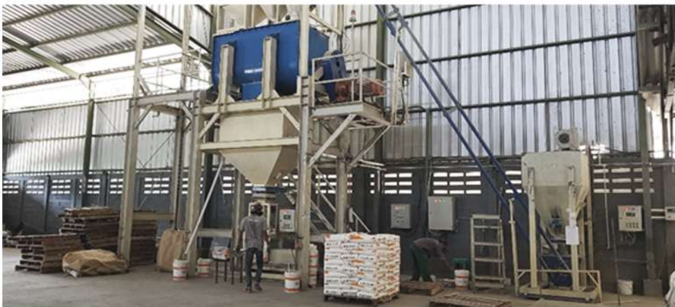
2 Ton Powder Mixer With 70 Ton per Shift Capacity
